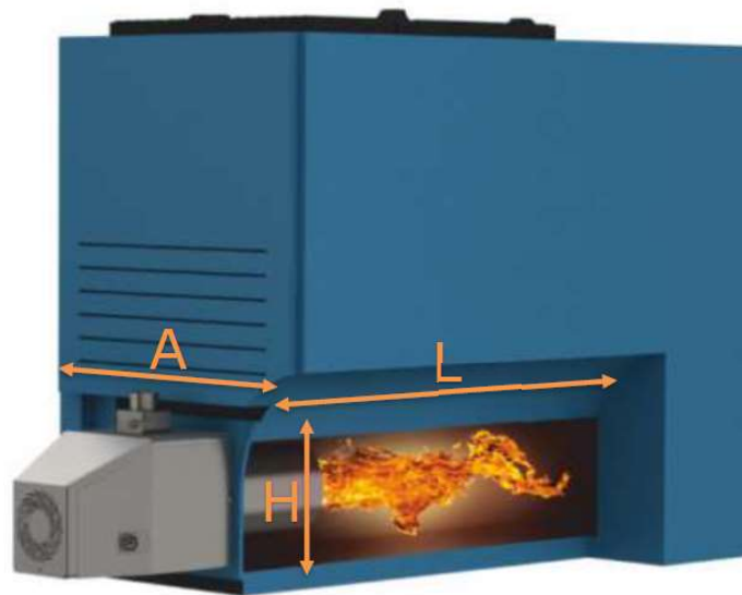
Fig. 3. Location of burner with respect to the direction of the flame.
